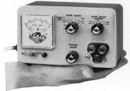
Fig. 1. —hp— Model 721A power supply provides 0 to 30 vdc at currents up to 150 ma. Maximum current available can be set by panel switch to minimize accidental overloading of sensitive external circuits.
